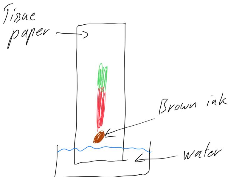
Put a spot of brown ink at the bottom of a piece of tissue paper and then dip the paper and water allowing the water to rise up the tissue paper. Observe the colors that are shown above the brown ink spot.
